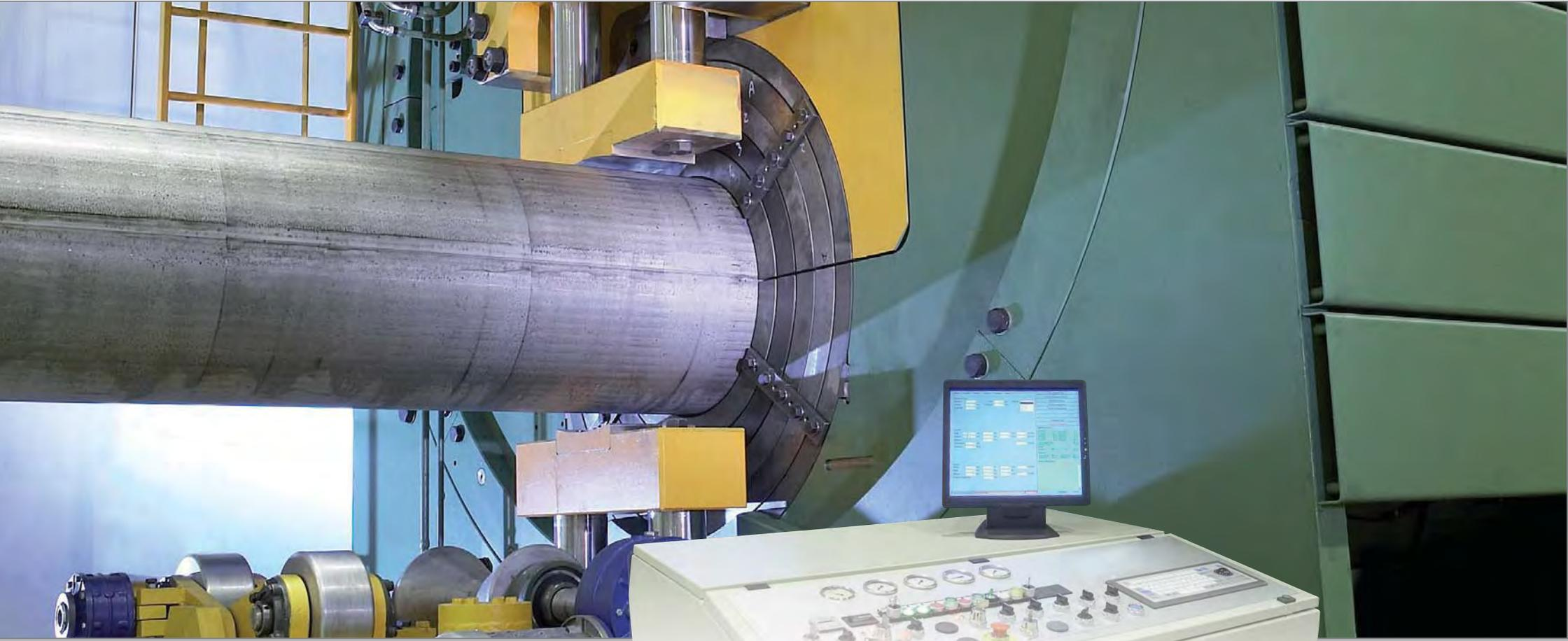
The calibration plant works the pipe to the dimensions and tolerances as required by the specification.
