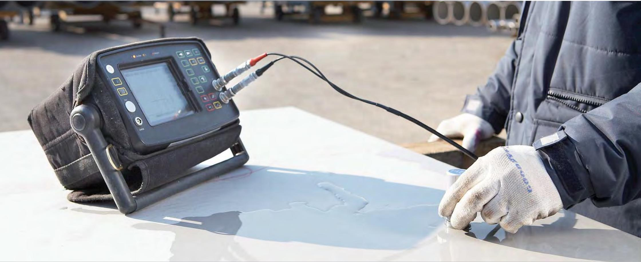
Raw material and consumables are purchased only from approved qualified suppliers. All incoming plates are inspected visually, dimensionally and PMI checked in order to fulfil the requirements of our internal procedures. When requested, before starting to work the raw material, further tests and verifications may be performed, including ultrasonic, hardness and dye penetrant tests. We also carry out random chemical analysis tests.
