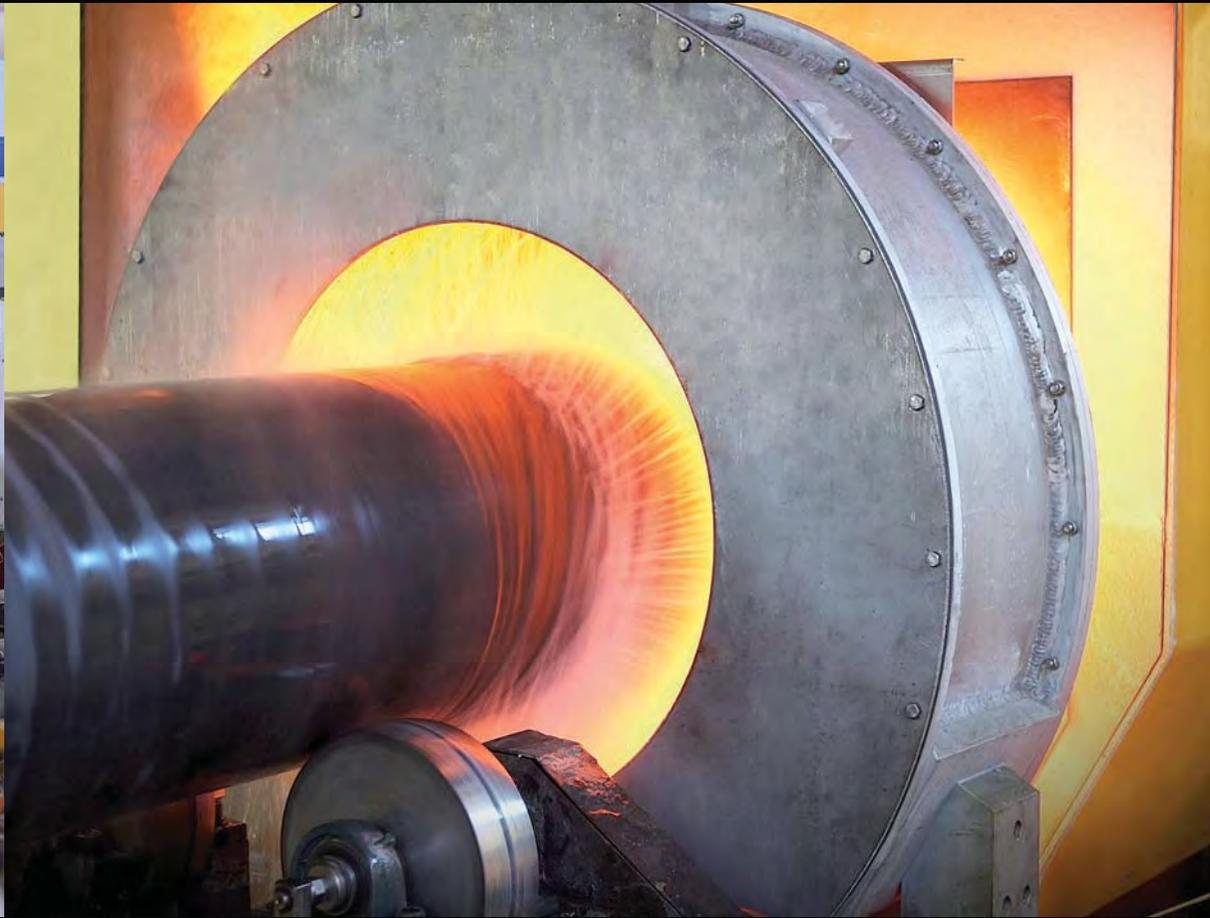
Rivit's heat treatment department has both induction and batch type furnaces which are calibrated in accordance with ASTM A 991 and API 5L for annealing and stabilising of all materials.
